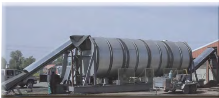
Drum composter - three day retention time.
